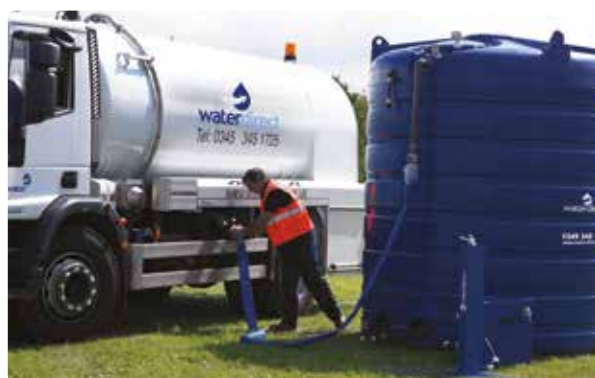
10,000 litre tanker pumping into a 10,000 litre static tank with quality assured water using five metres of 2" lay flat hose.
