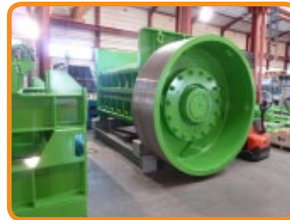
Images left show the BDR 2400 shredder in construction at Kemsley Mill, Kent and also at MTB's factory near Lyon, France.
